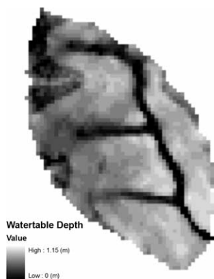
Fig. 4. Spatial water table depth (m) distribution for Slapton Wood, UK after 950 h of simulation, illustrating output options with OBJTOP.
