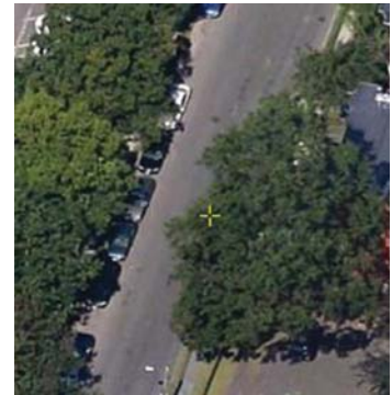
Photo-interpretation involves classifying randomly located points within preselected cover classes (e.g., tree, impervious, water).
