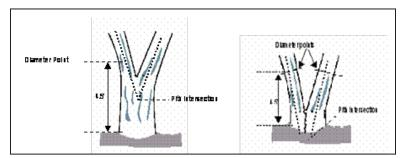
Fig. 7. Measuring DBH in forked (multistemmed) trees.
