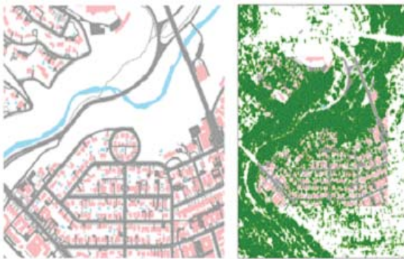
A planimetric map of a Washington DC neighborhood shows a neighborhood's gray infrastructure including buildings and roads (left). Classified high-resolution satellite imagery adds a green infrastructure data layer (trees and other vegetation) with its associated environmental benefits (right).
