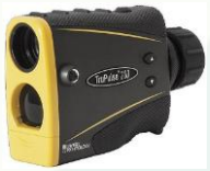
Laser Range finder (Height, Crown width)
