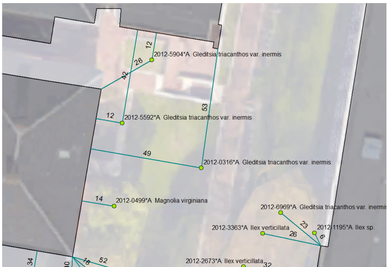
Figure 3: Distances in feet from tree center points to building polygons, as measured using ArcGIS. Trees are labeled by accession number and species. This is a close up of the music building courtyard and engineering quad. (Google Maps, 2015).
