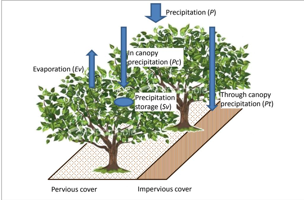
Figure 2 1<sup>st</sup> stage of the precipitation interception by vegetation, starting when the precipitation ( $P$ ) starts and ending when the canopy storage ( $Sv$ ) reaches  $Sv_{max}$
