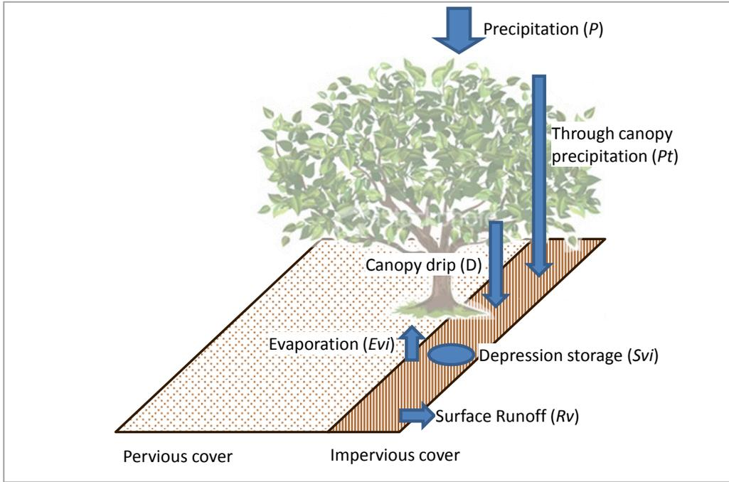
Figure 5 1<sup>st</sup> stage of the precipitation interception by impervious cover, starting when the precipitation ( $P$ ) starts and ending when the depression storage of impervious cover ( $Svi$ ) reaches  $Si_{max}$
