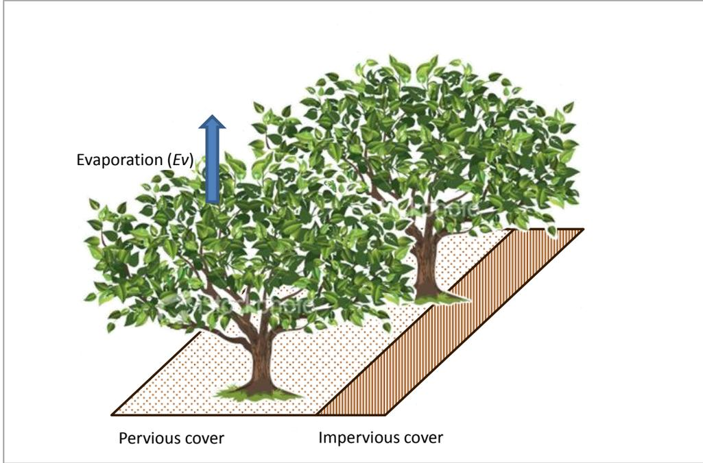
Figure 4 3<sup>rd</sup> stage of the precipitation interception by vegetation is drying stage, starting when precipitation stops
