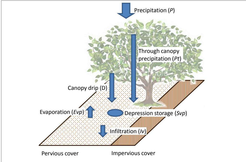
Figure 6 1<sup>st</sup> stage of the precipitation interception by pervious cover, starting when the precipitation ( $P$ ) starts and ending when the depression storage of pervious cover ( $Svp$ ) reaches  $Sp_{max}$
