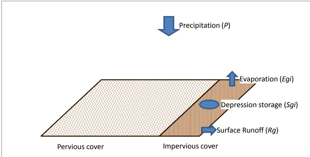
Figure 7 1<sup>st</sup> stage of the precipitation interception by impervious cover, starting when the precipitation ( $P$ ) starts and ending when the depression storage of impervious cover ( $Sgi$ ) reaches  $Si_{max}$
