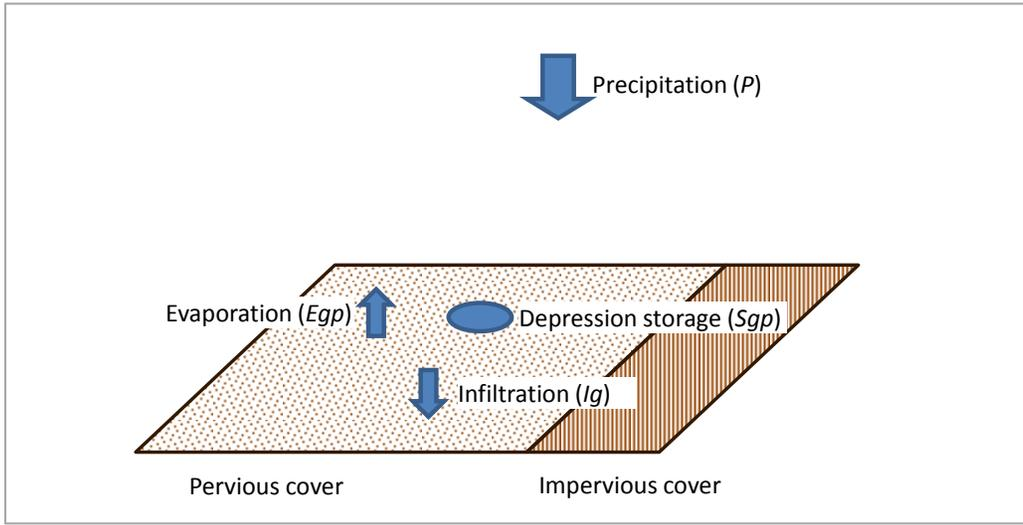
Figure 8 1<sup>st</sup> stage of the precipitation interception by pervious cover, starting when the precipitation ( $P$ ) starts and ending when the depression storage of pervious cover ( $S_{gp}$ ) reaches  $S_{p_{max}}$
