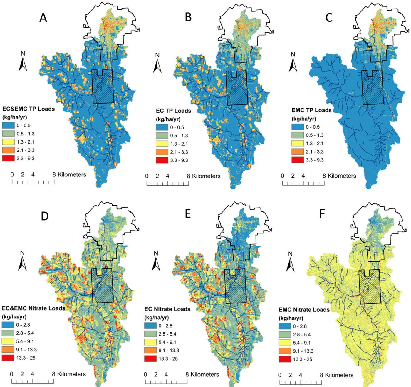
FIGURE 2. Demonstration of Using Export Coefficients and Event Mean Concentrations (EC&EMC), Only EC, and Only EMC to Determine Total Phosphorus (A-C) and Nitrate (D-F) Loads.
